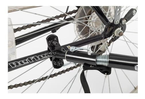
Wrap the securing strap around the frame as much as possible and attach the clip to the strap
