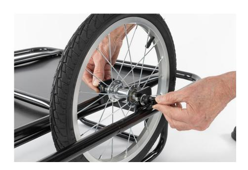
Screw the conical nut in a clockwise direction on to the quick release lever to secure it
