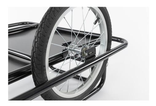
Place the locking washer onto the axle ensuring it is hooked into the hole in the axle
